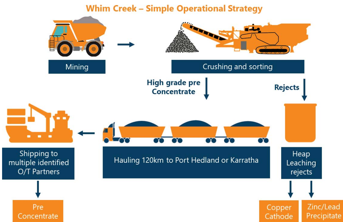
Figure 2: Smart Sorting Technology Enables Ore Processing to be Separated from Mining
