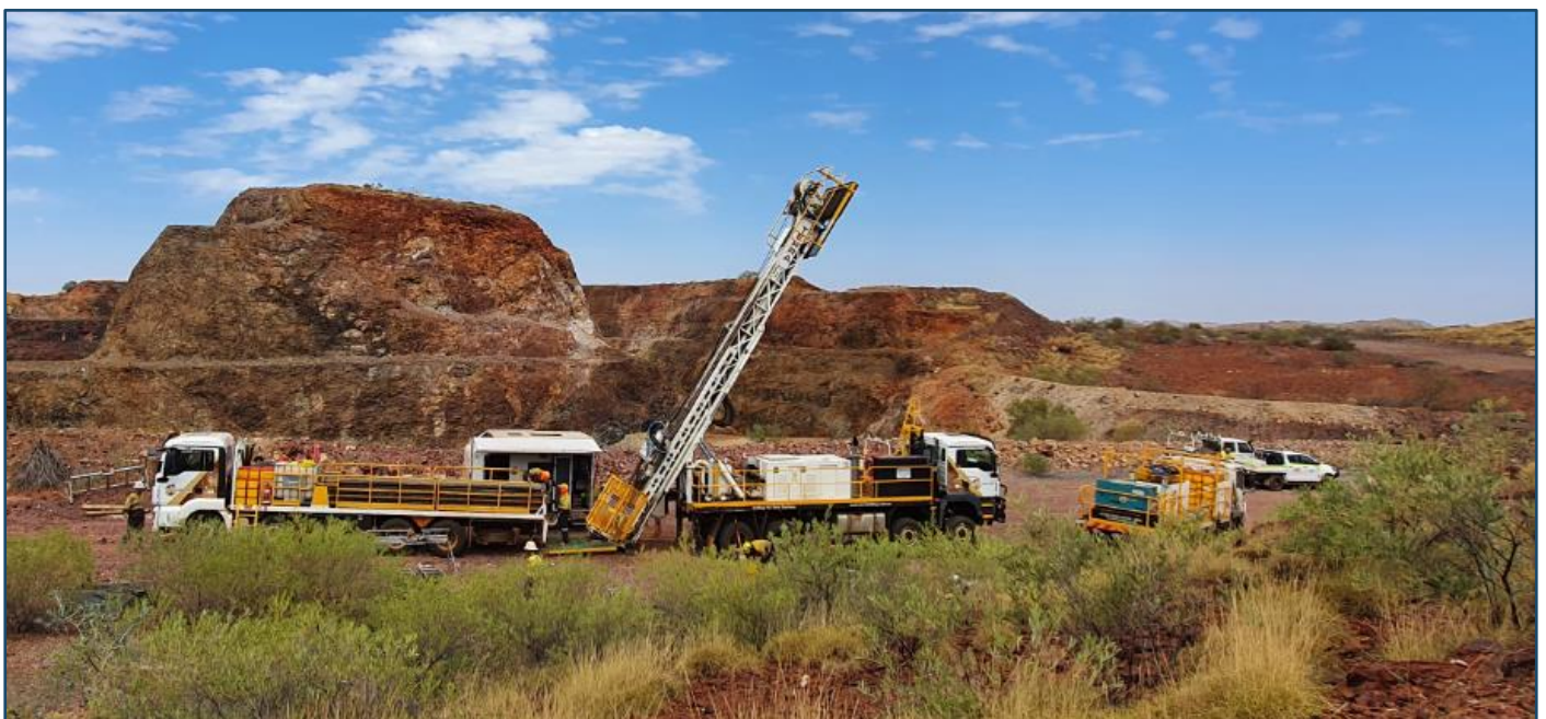
Image 1: Diamond Drilling at Mons Cupri, Whim Creek Project
