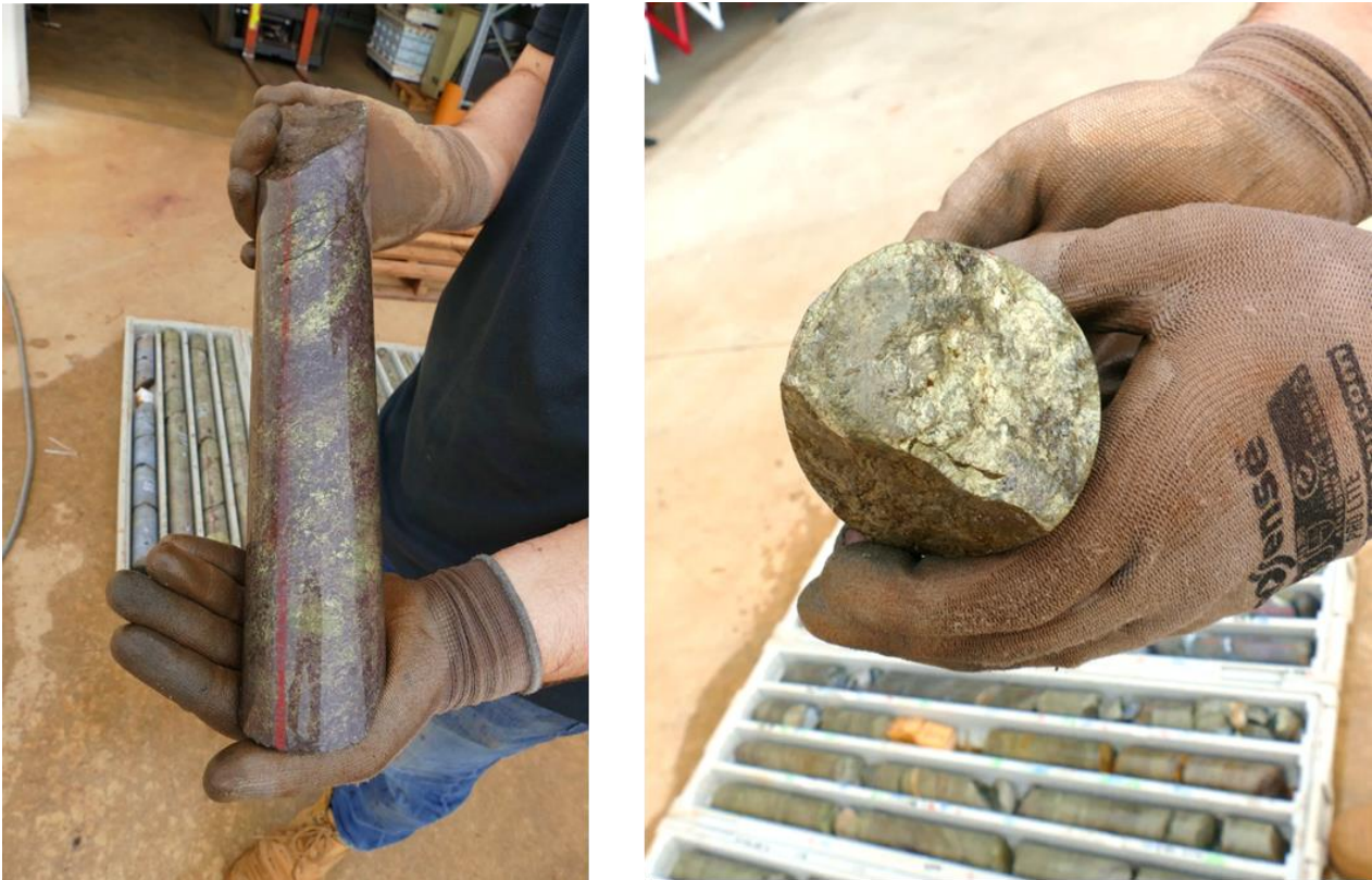
Figure 1: Massive sulphide copper-zinc mineralisation in 22AED003 and 22AED004A 2
