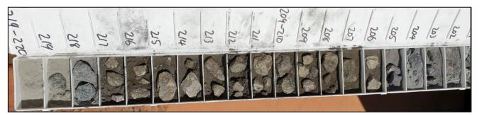
Figure 3: Chip tray showing massive sulphide copper-zinc mineralisation in 22AER005B
