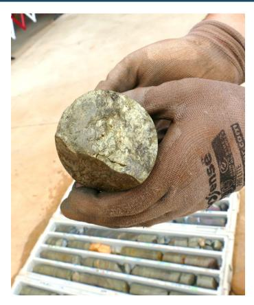
Figure 2: Massive sulphide copper-zinc mineralisation in 22AED003 and 22AED004A
