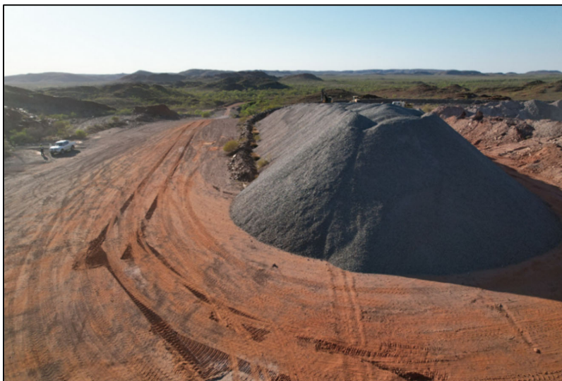
Figure 10: Commercial scale waste rock to road base trial product
